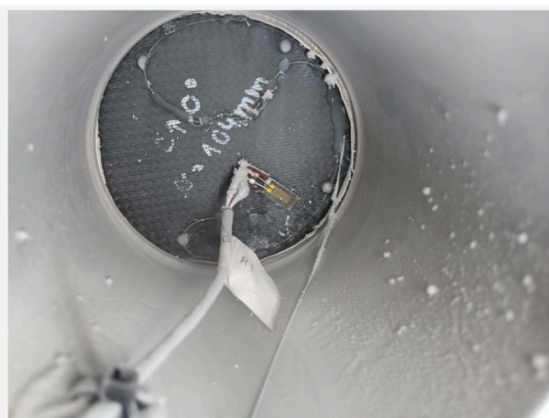
Fiber optic strain sensors surviving -196°C conditions.
